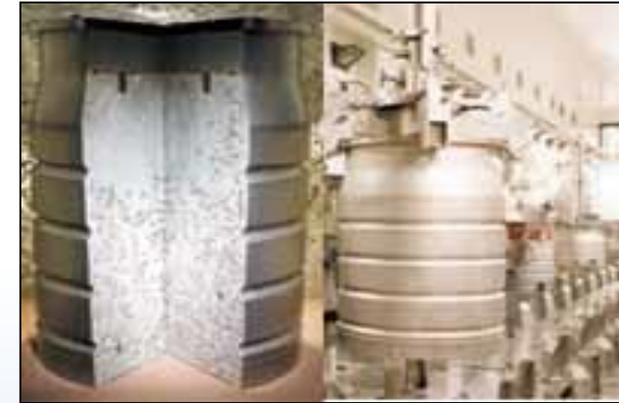
**ILW packed in cemented steel drum**
